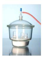
To open the stopcock, turn slightly; allow air to enter slowly. After pressure equalisation carefully push the lid until it moves.
